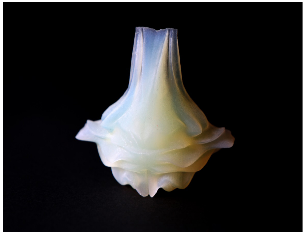
Fig. 8. Nose project Radiator / resonator – photo of 3D printed object in Flexible material Tango Plus 9740. Technology polyjet, solidified liquid photopolymer by using UV light (front view).
