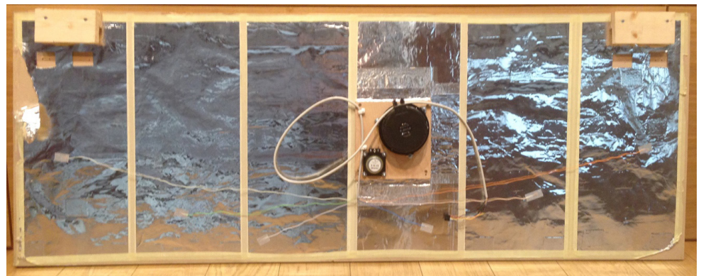
Fig. 2.2. Background view of an interactive panel: dual transducer assembly and six touch electrodes.
