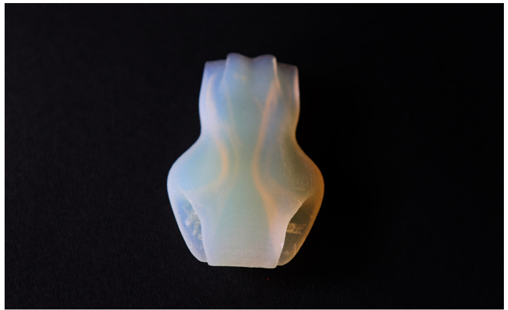
Fig. 6. Nose project Boxer —photo of 3D printed object in Flexible material Tango Plus 9740 . Technology polyjet, solidified liquid photopolymer by using UV light.
