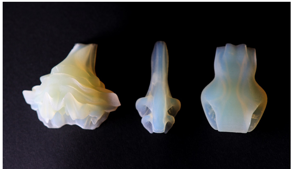
Fig. 15. All three selected models — photo of 3d printed object in Flexible material Tango Plus 9740. Technology polyjet, solidified liquid photopolymer by using UV light.
