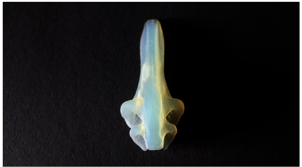
Fig. 4. Nose project Double nostrils – photo of 3D printed object in Flexible material Tango Plus 9740 . Technology polyjet, solidified liquid photopolymer by using UV light.
