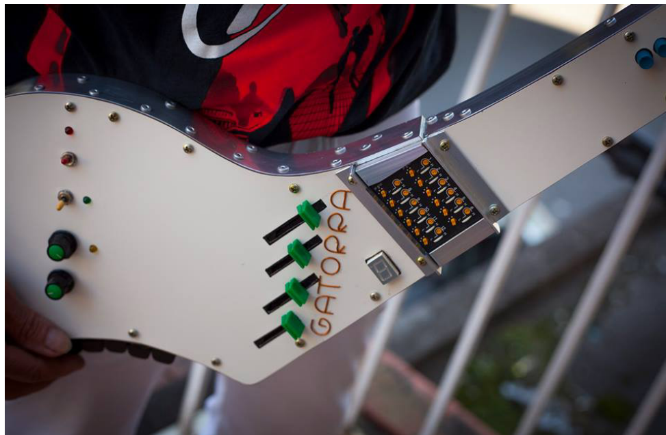
Fig. 5. Detail of Gatorra #3, equipped with a TV tuning panel.
